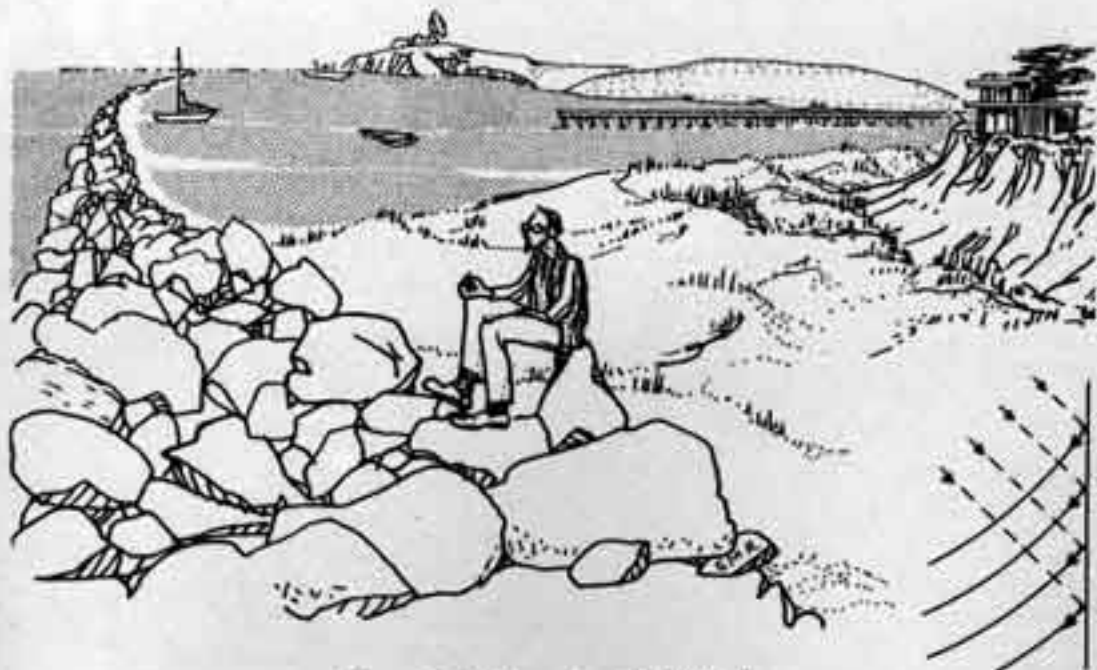
Figure 2. Half Moon Bay: BREAKWATER Diagram: Shows ocean waves from Alaska hitting coast & bouncing off at an angle.
